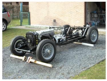
By the middle of the summer, the chassis, brakes, steering, and suspension were complete and the engine and gearbox were in.
